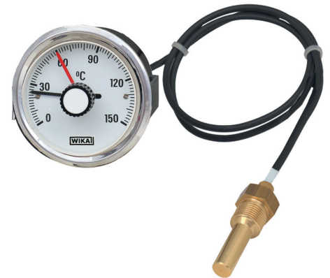
Chromated steel case with panel ring and clamp 1 adjustable change over switch Plastic coated capillary Rotable connection with thermowell of brass L-45 mm G1/2"
